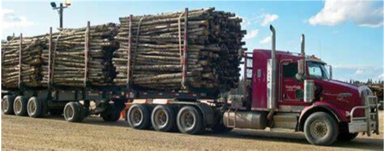
Example of a truck with a hay rack configuration. More racks may be required depending on the size of the woody material being hauled. (Photo credit: https://forestnet.com/LSissues/July_10/alberta1.jpg )
