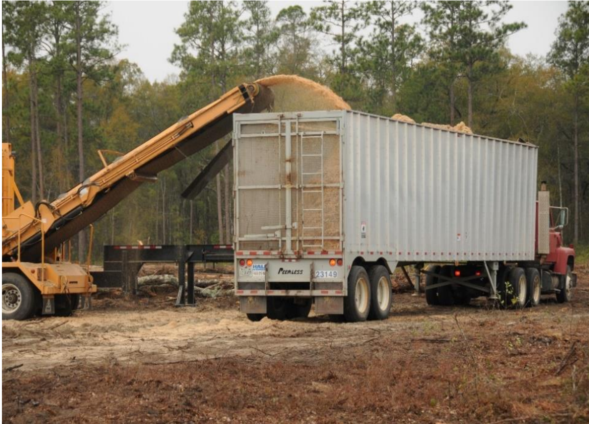
Example of loading ground/ chipped material in the bush, on easy, accessible ground. Photo credit: https://api.army.mil/e2/c/images/2012/02/02/233923/original.jpg
